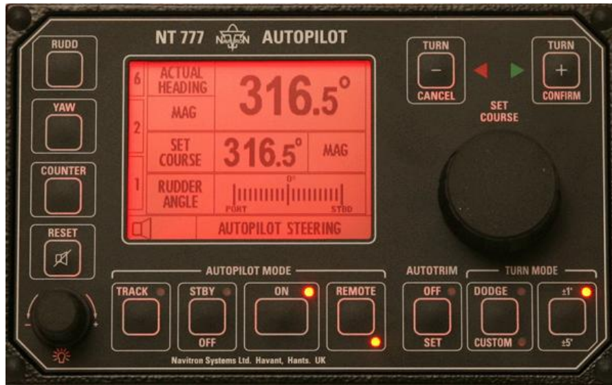
Model NT777 Autopilot Control Unit (192 x 120 x 62.4mm)
